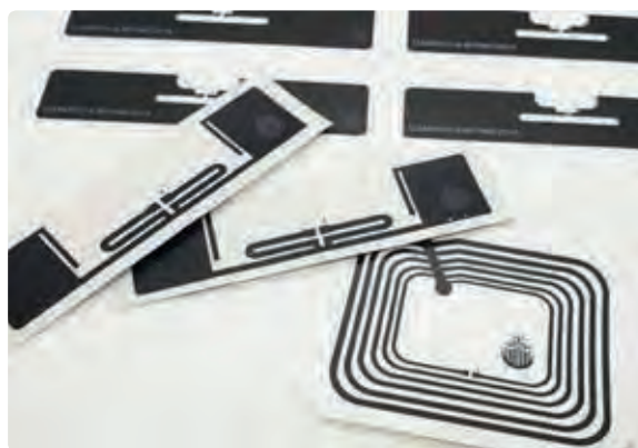
Radio Frequency Identification (RFID) Prototype Made from Conductive Ink and Transparent Conductive Film.
